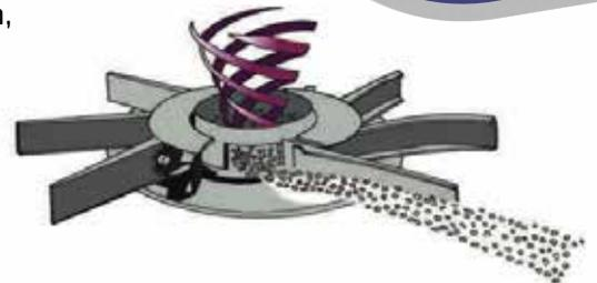
The Helix Duo precision system with a central chamber allows for smoother flow, leading to distribution with less dust and saving fertilizers/seeds.
